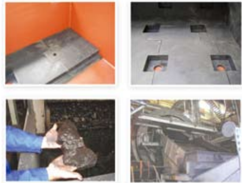
漏斗、溜槽的超耐磨橡胶衬板 Super anti-abrasion rubber liner of funnels and chutes
